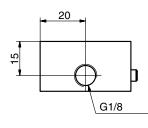
RR connection for blow off signal or the connection of other equipment.
