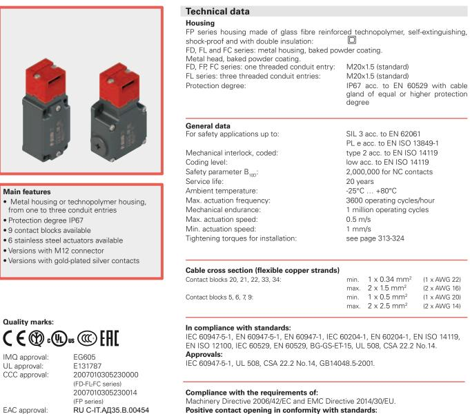
Positive contact opening in conformity with standards: IEC 60947-5-1, EN 60947-5-1
