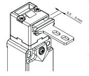
The actuation head of this switch features a wide range of travel. In this way the guard can oscillate along the direction of insertion (4.5 mm) without causing unwanted machine shutdowns. This wide range of travel is available in all actuators in order to ensure maximum device reliability.
