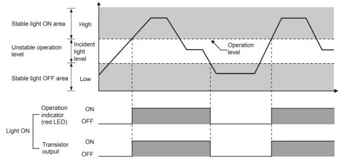
\*The waveforms of 'Operation indicator' and 'Transistor output' are for Light ON, it is operated as reverse in Dark ON.
