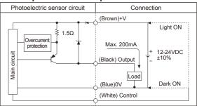
\*\*Select Light ON / Dark ON by control wire. - Light ON: Connect control wire to +V / Dark ON: Connect control wire to 0V
