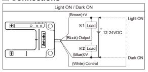
X1: Load connection for NPN open collector outputX2: Load connection for PNP open collector output
